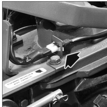
Figure 4-6: Plug and receptacle of Forward Interlock Safety System must be securely connected.
