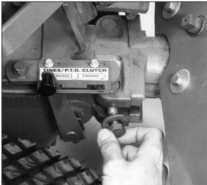
Figure 4-25: Moving swing-bolts outward.
