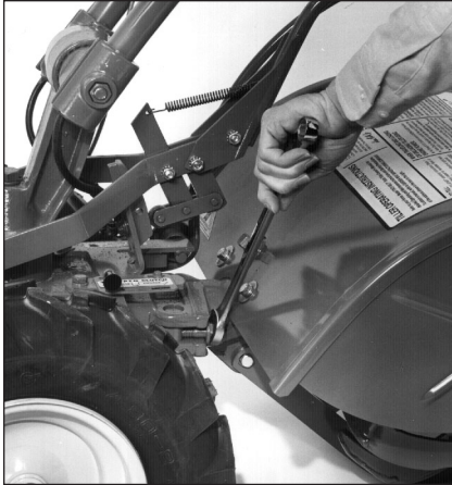
Figure 4-24: Loosening attachment swing-bolts.
