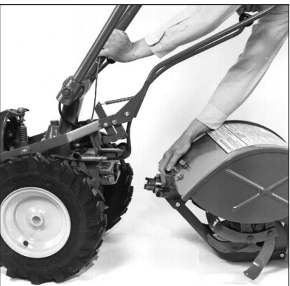
Figure 4-26: Pulling attachment away from power unit.
