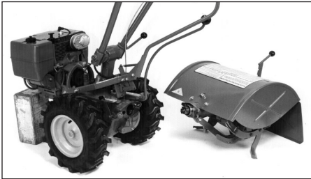
Figure 4-21: PTO Power Unit and tine attachment.
