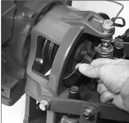
Figure 5-19: Move top half of belt over pulley and reverse disc.
