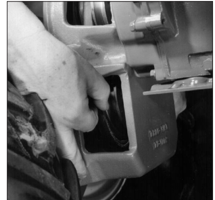
Figure 5-17: First move belt off the lower pulley.
