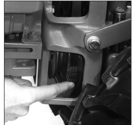
Figure 4-13: High range to low range. Shows moving belt from lower-front onto lower-rear groove.
