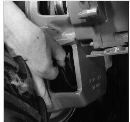
Figure 5-17: First move belt off the lower pulley.
