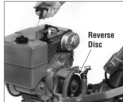
Figure 5-25: Checking Reverse Disc in NEUTRAL.
