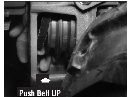
Figure 5-18: Push belt upward to create slack.
