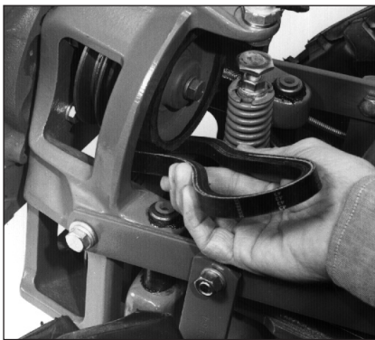
Figure 5-20: Shift into FORWARD and remove the belt.
