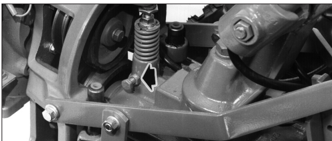
Figure 5-2: Check jam nut on plunger assembly.
