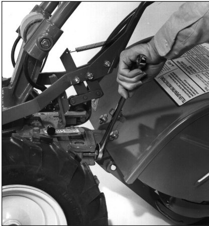
Figure 4-24: Loosening attachment swing-bolts.
