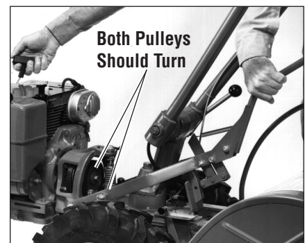
Figure 5-26: Checking Reverse Disc in REVERSE.
