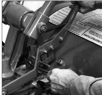
Figure 5-16: Hold Drive Lever while loosening bolt. Push lever down to tighten belt; pull up to loosen belt.
