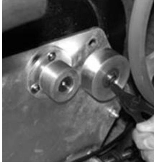
Step 2. Remove Snap Ring
