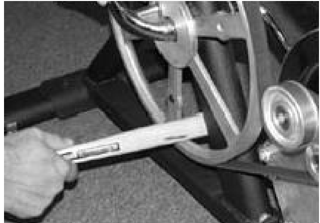
Step 1. Prevent Rotation of Fly Wheel
