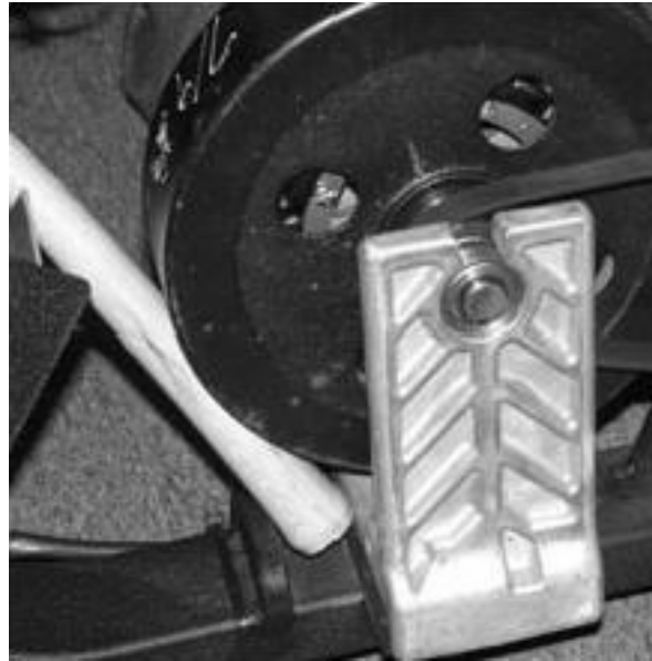
Step 3. Pry on Brake to Loosen Belt.
