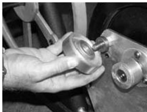
Step 7. Remove belt tensioner
