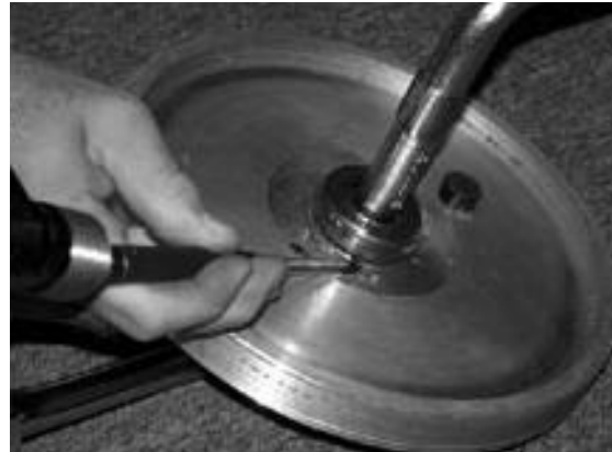
Step 7. Drive Spanner Nut Off to Remove Bearing
