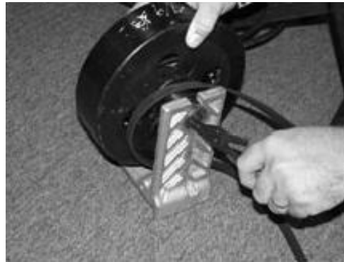
Step 1. Remove Snap Ring.
