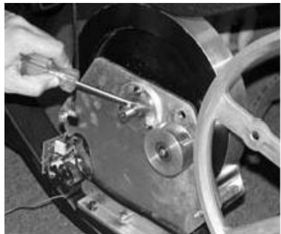
Step 2. Remove Keyway
