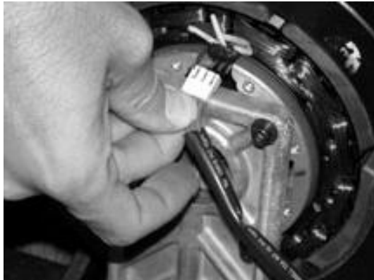
Step 5. Disconnect Wiring Harness.
