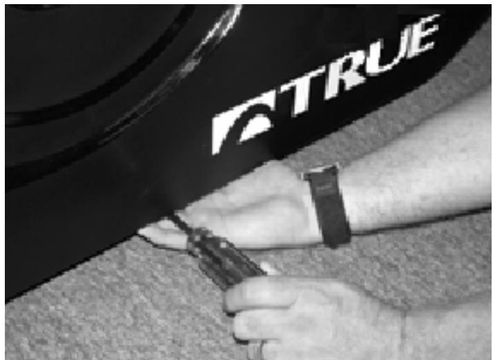
Step 2. Remove Cover Screws
