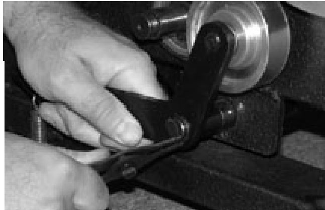
Step 1. Remove Snap Ring
