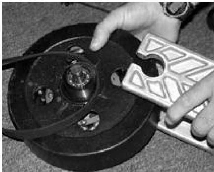
Step 5. Remove Bracket to Check Belt
