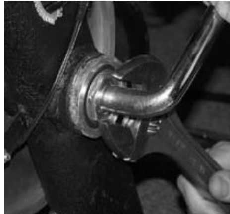
Step 4. Pull Hex Nut Bearing Free.
