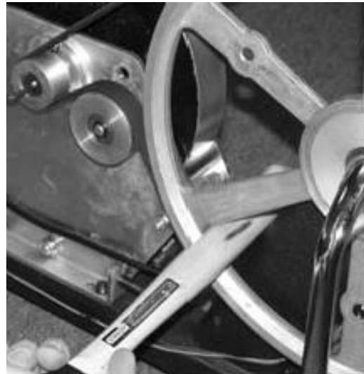
Step 1. Prevent Rotation of Fly Wheel
