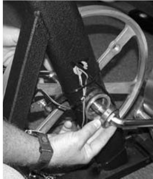
Step 4. Pull Hex Nut Bearing Free
