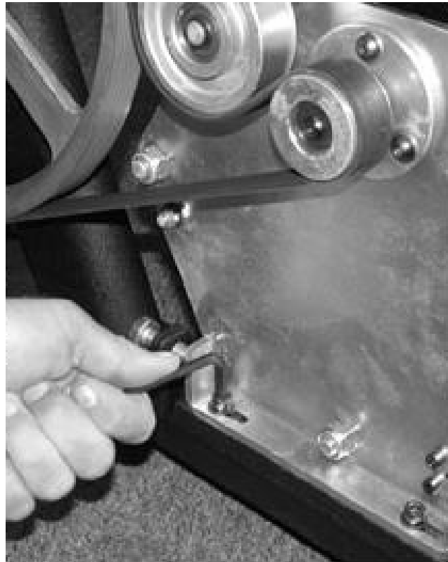
Step 4. Loosen setscrew
