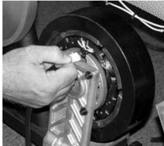
Step 5. Disconnect Wiring Harness.
