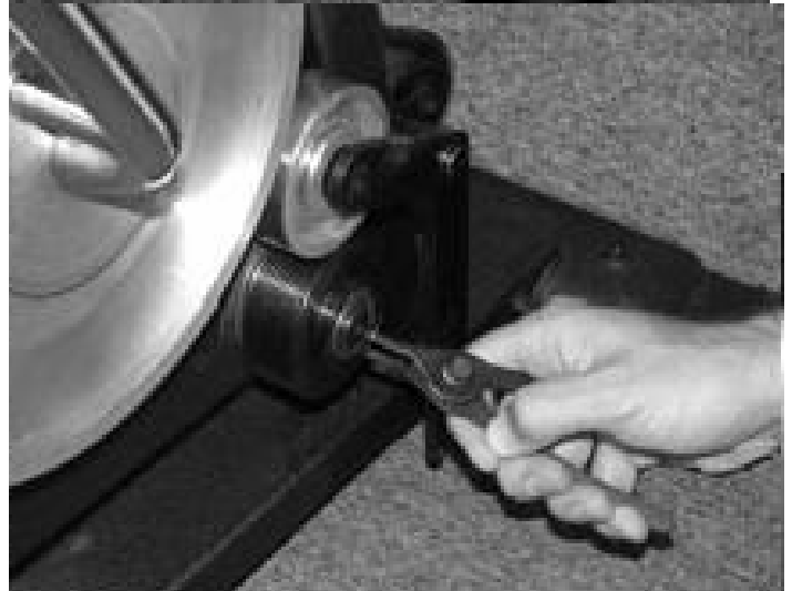
Step 1. Prying with Snap Ring Pliers.
