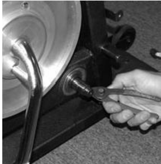
Step 1. Remove Shaft Snap Ring on Right Side
