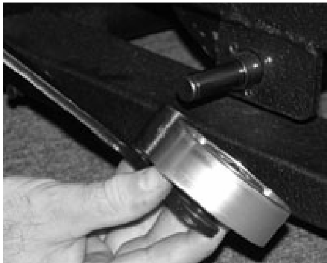
Step 2. Slide Tensioner Assembly
