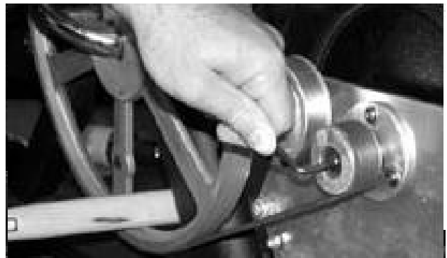
Step 2. Loosen Set Screw
