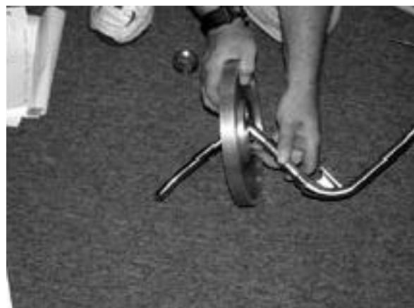
Step 9. Pull Crank Thru Pulley to Remove
