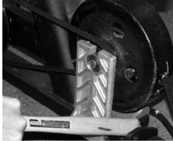
Step 3. Pry on Brake to Loosen Belt.
