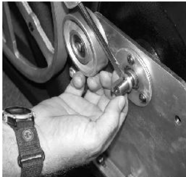
Step 2. Remove keyway
