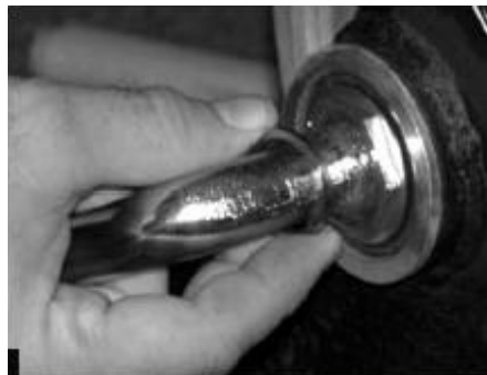
Step 2. Remove Keyed Washer
