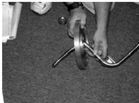
Step 9. Pull Crank Thru Pulley to Remove
