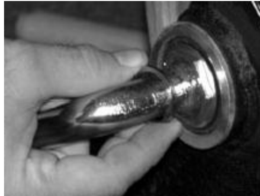
Step 2. Remove Keyed Washer
