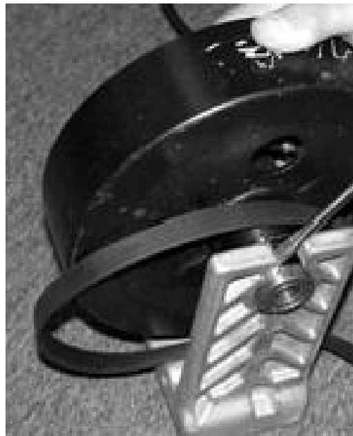
Step 2. Pry Bearing Out of Housing
