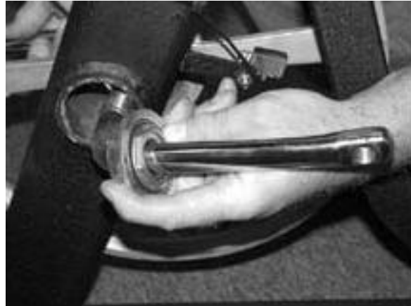
Step 4. Pull Hex Nut Bearing Free.
