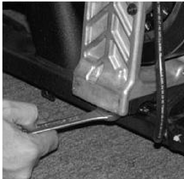
Step 2. Loosen Bracket Bolts
