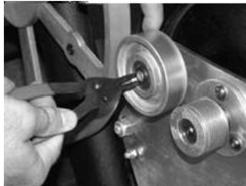
Step 6. Remove Snap Ring.
