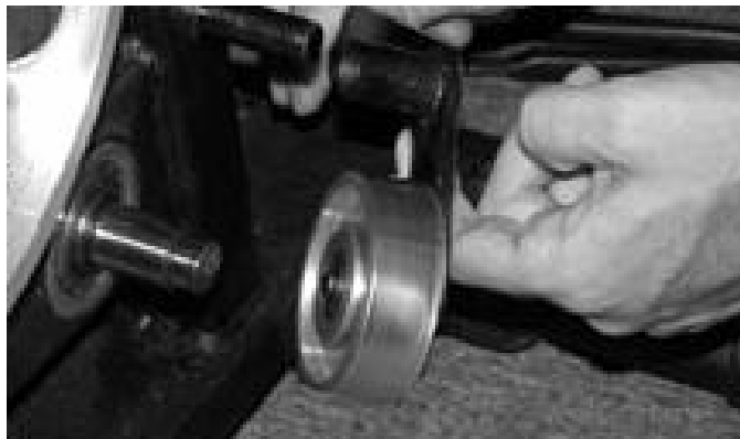
Step 2. Slide Tensioner Assembly
