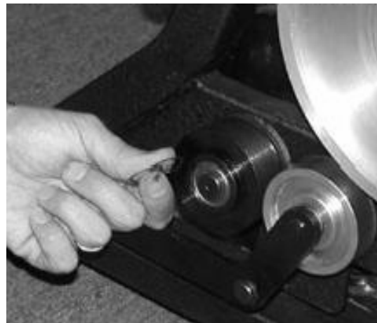
Step 4. Remove the snap ring and washers
