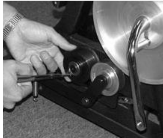
Step 3. Prying with snap ring pliers
