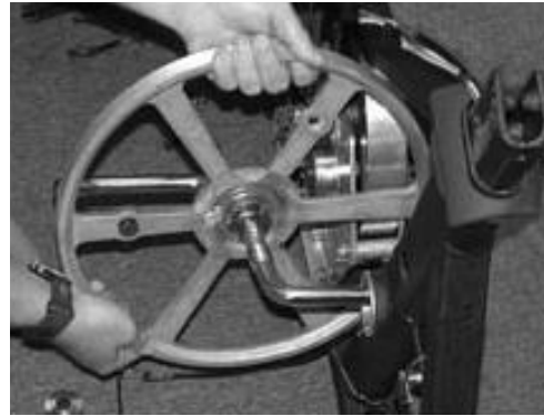
Step 6. Twist Unit Thru Hub Frame
