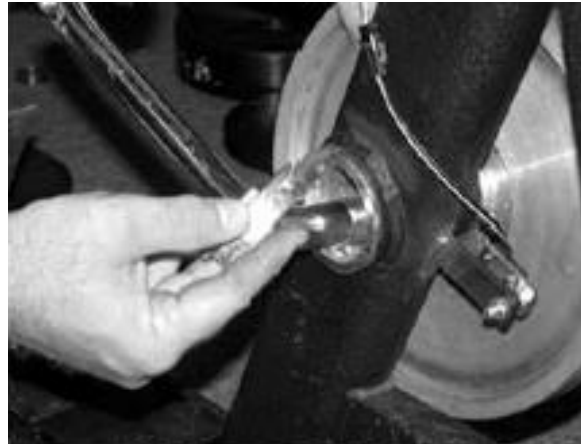
Step 4. Pull Hex Nut Bearing Free.
