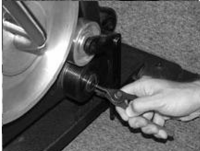
Step 1. Remove Snap Ring
