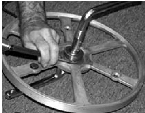
Step 7. Drive Spanner Nut Off to Remove Bearing
