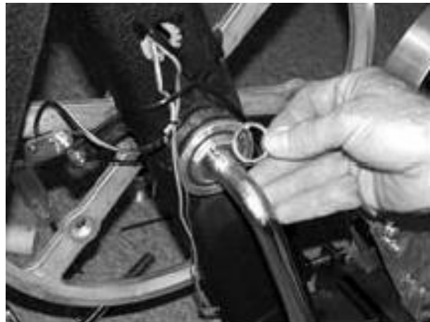
Step 2. Remove Keyed Washer
