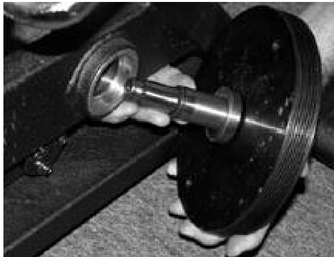
Step 2. Slide Shaft Through Frame
