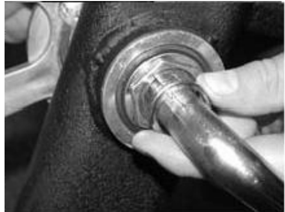
Step 2. Remove Keyed Washer
