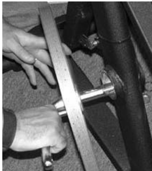
Step 4. Pull Hex Nut Bearing Free.
