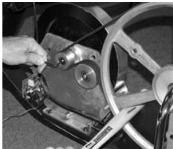
Step 2. Loosen Set Screw
