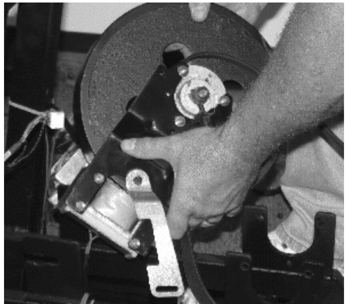
Step 5. Lift Brake & Magnet Assembly Out.
