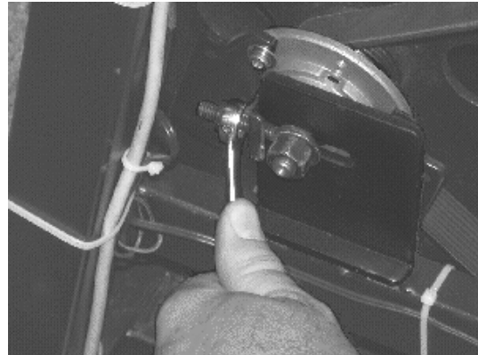
Step 1. Loosen Belt Tensioning Nuts.
