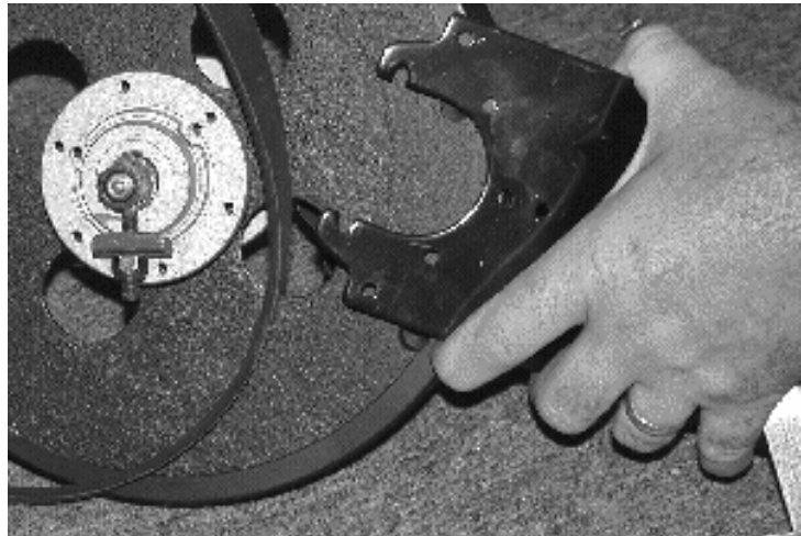
Step 7. Remove Brake Brackets & Belt.
