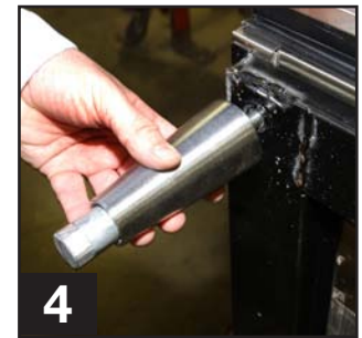
4 Thread leg into cabinet bottom frame rail.
