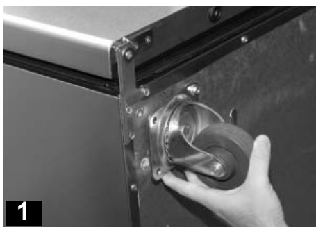
1 Thread four screws into castor in the underside of cabinet frame rail.
