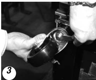
3 Use the tool provided to tighten the castor into place.
