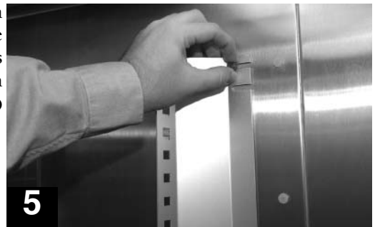
Pilaster Installation Two and Three Door Models (Middle of Wall in Rear of Cabinet)
