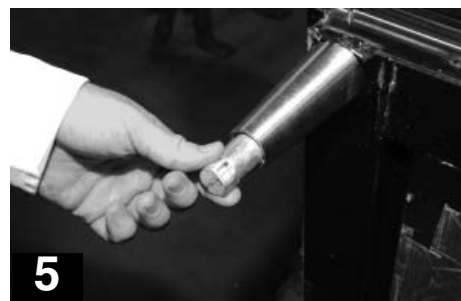
5 The end of the leg is adjustable to easy leveling.
