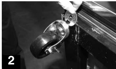
2 For leveling, insert the shim between the castor and frame rail.
