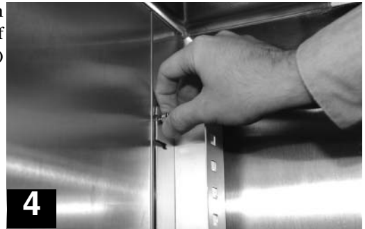
Pilaster Installation (Side Wall of Cabinet)
