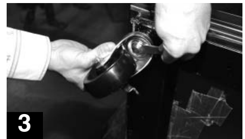
3 Use the tool provided to tighten the castor into place.
