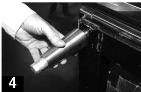
4 Thread leg into cabinet bottom frame rail.
