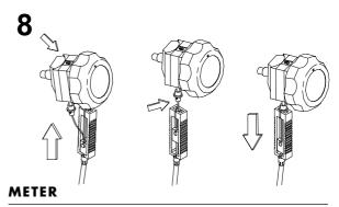
Pop open the battery cover at the back of the meter to assemble batteries. Close the cover. Remove the cable ties from the wires of the handlebar support. Connect the wires to the respective connectors on the meter and then thread the wires into the handlebar. Be careful not to damage the wires when attaching the interface. Slide the meter on the top of the handlebar support tube and attach it with three locking screws through the plastic sleeve.
