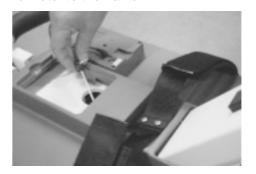
Support the rail with one hand, place the fastening screws and sleeves through the holes in the rail, and screw, finger-tight only, into the threaded holes in the frame.
