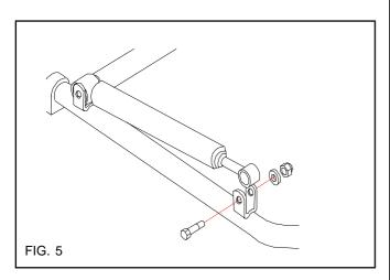
Remove the plastic cover on the bearing housing of the oar. Make sure that the sleeve bearing remains inside the bearing housing. To install the oar, place its lower end in the oar bracket, push the screw through the bracket and the sleeve (fig. 6). Insert the washer and tighten the nut, holding the bolt in place with an open-end wrench. Tighten the screw hard. Install the other oar in the same manner.
