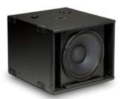
It consists of a single 15" reflex-loaded low frequency driver in an optimally tuned 18mm (3/4") birch plywood enclosure with built-in pole mount socket and moulded corner protectors. Two Speakon NL4 connectors provide input and link out connections.
