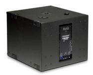
It consists of one 15" reflex-loaded low frequency driver in an optimally tuned enclosure with pole mount socket and moulded corner mouldings constructed from 18mm (3/4") birch plywood and incorporating an integrated Class D amplifier and control electronics module. The rear panel carries input and link XLRs, RJ485 network connectors, low frequency contour, power switch and status LED's.
