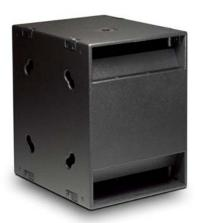
It consists of a single 18" bandpass-loaded low frequency driver in an optimally tuned 18mm (3/4") birch plywood enclosure with pole mount socket constructed from with a built-in pole mount socket and moulded corner protectors. Two Speakon NL4 connectors provide input and link out connections.
