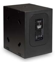
It consists of one 18" bandpass-loaded low frequency driver in an optimally tuned enclosure with pole mount socket and moulded corner protaectors constructed from 18mm (3/4") birch plywood and incorporating an integrated Class D amplifier and control electronics module. He rear panel carries input and link XLRs, RJ485 network connectors, low frequency contour, power switch and status LED's.
