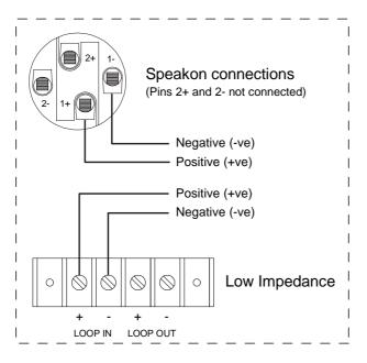
Note that looping out to additional enclosures has the effect of reducing the load impedance on the amplifier. For example, two 8 ohm cabinets in parallel give a combined total impedance of 4 ohms. Never connect loudspeakers whose total combined impedance is lower than the amplifier's recommended minimum load impedance. Do not use the loop-out connection to connect other types of loudspeaker, especially when their impedance is not known, as permanent damage could result!
