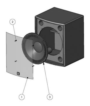
The perforated steel loudspeaker grille (1) is held in place under tension only, fitting into slots at either side of the baffle. There are no screws or other fixings holding the grille in place. Lay the cabinet on its back and, using two small screwdrivers inserted through the mesh of the grille, firmly pull the grille away from the slot at one side of the baffle until it is free. Set the grille aside for later re-assembly.
