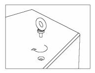
As supplied, these rigging points are fitted externally with M10 countersunk slot-head screws. To facilitate rigging of the enclosure simply remove these M10 screws and replace them with M10 x 18mm shoulder eyebolts using a suitable thread locking compound to avoid the possibility of loosening.
