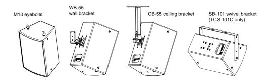
All TCS COMPACT series cabinets, including low frequency enclosures, can be rigged in permanent installations using optional M10 shoulder eyebolts (available from Turbosound or third party suppliers). These can be attached to the rigging points provided on the top and back of the cabinet. The rigging point at the rear of the cabinet is used to alter the downward angle of the enclosure.
