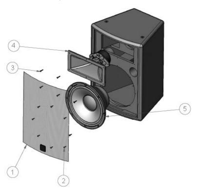
The perforated steel loudspeaker grille (1) is held in place under tension only, fitting into slots at either side of the baffle. There are no screws or other fixings holding the grille in place. Lay the cabinet on its back and, using two small screwdrivers inserted through the mesh of the grille, firmly pull the grille away from the slot at one side of the baffle until it is free. Set the grille aside for later re-assembly.
