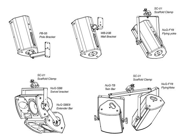
To install a loudspeaker using Turbosound brackets, first separate the brackets into their wall/ceiling plate and speaker plate component parts. Remove the two countersunk M10 bolts on the rear panel of the cabinet. Attach the speaker plate to the cabinet with the M8 bolts supplied. Fix the wall/ceiling plate in the venue using appropriate fixings (not supplied). Lift the loudspeaker on to the wall plate and re-assemble the bracket parts, adjust the vertical angle and tighten all bolts.
