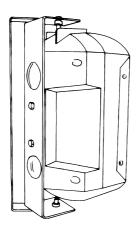
Fixing to a wall or ceiling using the **SB-50** swivel bracket. When used vertically as shown attached to a wall, the enclosure is free to rotate in the horizontal plane over more than 180°. It can also be turned through 90° and mounted horizontally on to a wall in which case the enclosure can be tilted downwards to give the desired coverage. The SB-50 can also be fixed to a ceiling, again allowing for a wide range of adjustment of the enclosure.
