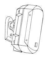
Attaching to a scaffold bar or to a microphone stand by means of the **SM-50** single point mount bracket. For microphone stand use simply remove the microphone clip from the mic stand and locate the threaded end through the hole in the top of the SM-50 bracket. Tighten with the wing nut provided. For use with a scaffold bar, place the bracket over the bar and tighten with the supplied M6 screw until secure.
