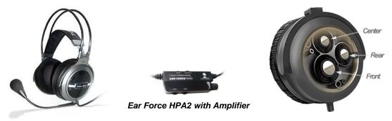
The headset includes four speakers in each ear cup for reproducing Front, Surround, Center and Sub audio signals from the Riviera 5.1 analog outputs, providing a realistic surround-sound experience without the need for a 5.1 speaker system.
