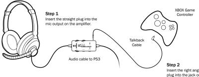
Insert the right angle plug into the jack on the XBOX controller.
