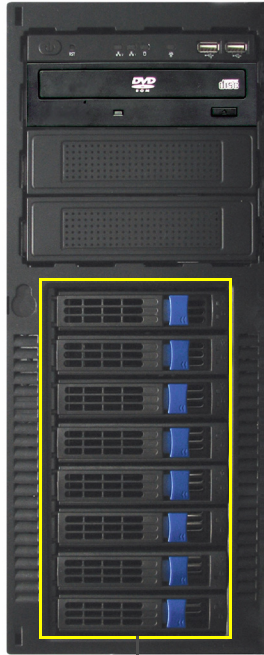
Hotswap HDD bays (Bottom to top: HDD1, HDD2, HDD3, HDD4, HDD5, HDD6, HDD7, HDD8)
