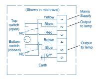
Low profile switchbox with Option 1 two V9 single pole double throw microswitches
