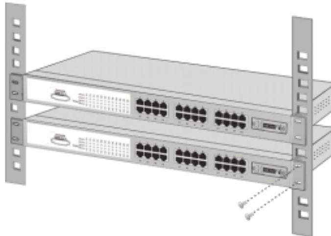
Figure 2-5. Mount the SmartGST-2402M in a standard 19-inch Rack
