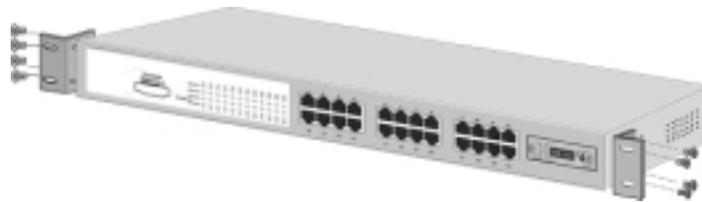
Figure 2-4. Attach mounting brackets with screws
