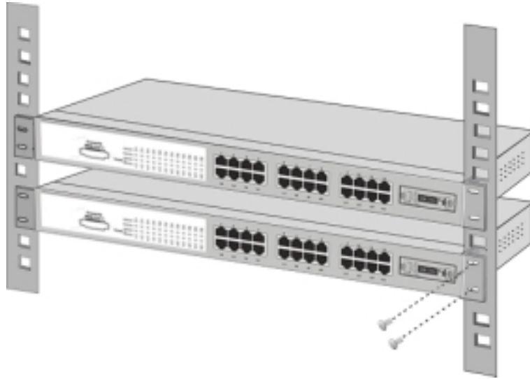
Figure 2-5. Mounting the Switch in an EIA standard 19" Rack
