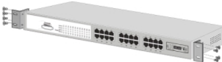
Figure 2-4. Attach mounting brackets with screws
