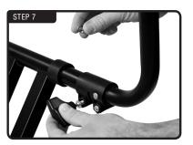
Install hand z-knob, washer, and hex nut. It is important to place the hand knob on the inside or stand will not fold fully. Also, be careful not to over-tighten the hand knobs because over-tightening may case cracking of the collar.
