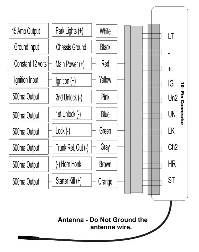
\*\*\*500ma outputs are low current and are designed to activate relays.
