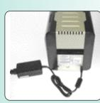
the rear). With AC power connected, the action of inserting the DC connector will switch on the Alto, and motor noises will be heard as the dyefilm panels are positioned, followed by the illumination of the green LED on the front panel. Your printer is now ready.
