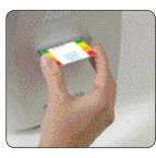
aperture on the front panel until resistance is felt. When the printer is ready to print, the LED will again flash, together with motor noise, and the card should be drawn into the printer and a test card printed. Note: If a subsequent test card is initiated, the image will
