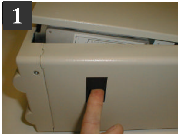
1 Open the Printer Top Cover by releasing the catch on the right-hand side of the printer.
