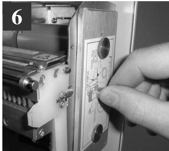
6 Turn the 'Dzus' Fastener 1/4 turn clockwise to lock in place. Lay the ring flat against the panel
