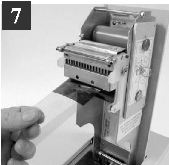
7 Pull about 6" of dye film off the roll of dye film, observing that it should be coming off the top of the roll, as per the label illustrations.
