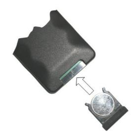
NOTE: Remove the battery if the remote control will not be used for a long time.
