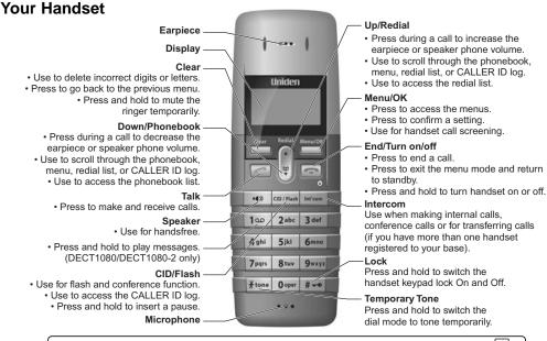
Note: Each handset can be turned off to conserve battery life. To turn off the handset, press and hold when the handset is turned off, you cannot make or receive calls on that handset. To turn the handset on again, press and hold or place the handset in the charger.
