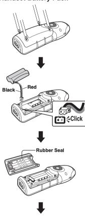
5) Insert the bottom end of the cover into the grooves on the handset and lay the cover over the battery compartment. Tighten the four screws securely.
