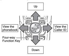
To use this four-way key, place your thumb over the key on the handset and move to the four positions to get the feel of how it moves and operates.
