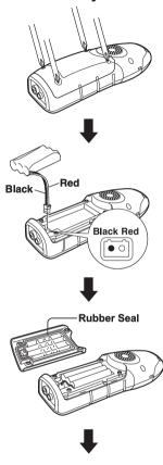
5) Insert the bottom end of the cover into the grooves on the handset and lay the cover over the battery compartment. Tighten the four screws securely.
