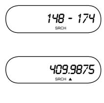
When **BAND** is pressed, this screen displays the band range to be searched. Press **BAND** again (or **UP/DOWN** within 3 seconds) to see other band ranges.
