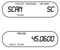
This screen shows BC355C is actively scanning a displayed bank. "SCAN" scrolls from right to left across the screen, and the scanned bank will flash.
