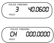
The screen cycles between two displays. The first screen shows that channel 3 on the **POLICE** bank (40.0600) is selected and the second screen shows that the null frequency (000.0000) is ready to be programmed.
