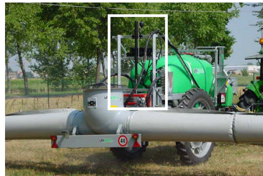
Lifting and Self-levelling system
