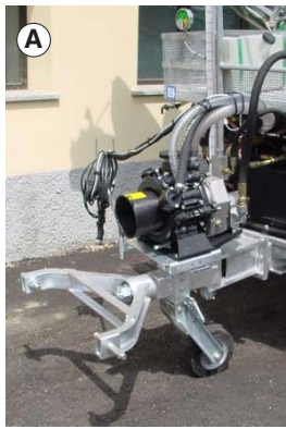
Tractor coupling for Towed machines: - (A) standard version, with elevator coupling - (B) homologated version, coupled to tow hook
