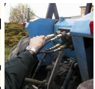
Elettrol connection to quick-fit couplings of the tractor
