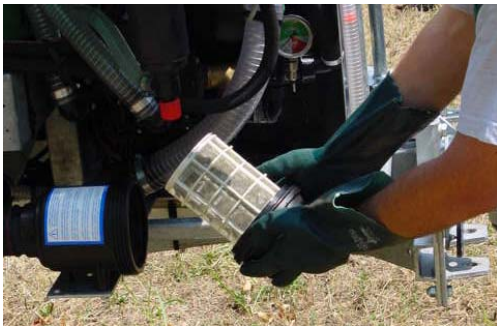
Dismantling the Suction Filter
