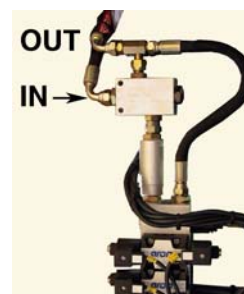
Elettrol connection to quick-fit couplings of the tractor
