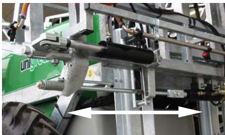
Self-levelling blocking system
