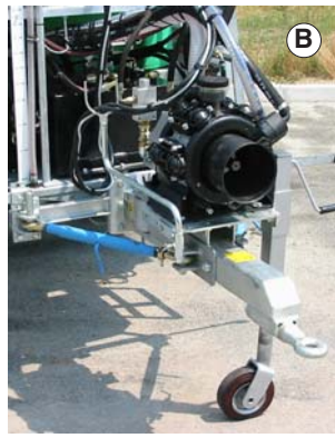
Tractor coupling for Towed machines: - (A) standard version, with elevator coupling - (B) homologated version, coupled to tow hook
