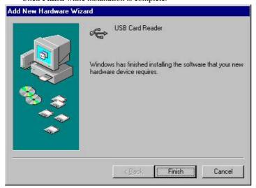
f. After installing, the System will generate an additional COM Port, USB Card Reader (e.g.: COM3) for the connection to RS232 Serial Device.
