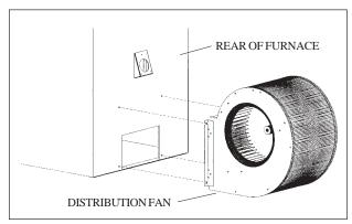
2. Attaching the distribution fan. First, remove the four (4) bolts from the rear of the unit. Secondly, slide the distribution fan up to the rear of the furnace, line up the (4) holes and reattach the bolts and tighten securely.
