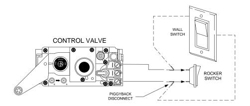
Remember the Rocker Switch must be turned to "OFF" while using the Wall Switch.
