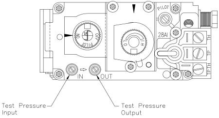
FIGURE 7. Pressure Test Point Location
