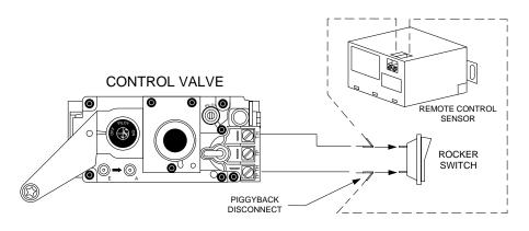
Remember the Rocker Switch must be turned to "OFF" while using the Remote Control.
