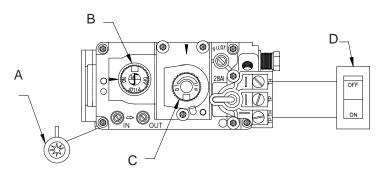
NOTE: Knob cannot be turned from "PILOT" to "OFF" unless knob is pushed in slightly. Do not force.
