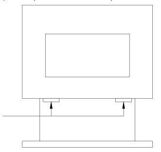
The 6035 has (2) front cleanout slides that must be in the closed position when burning the unit.
