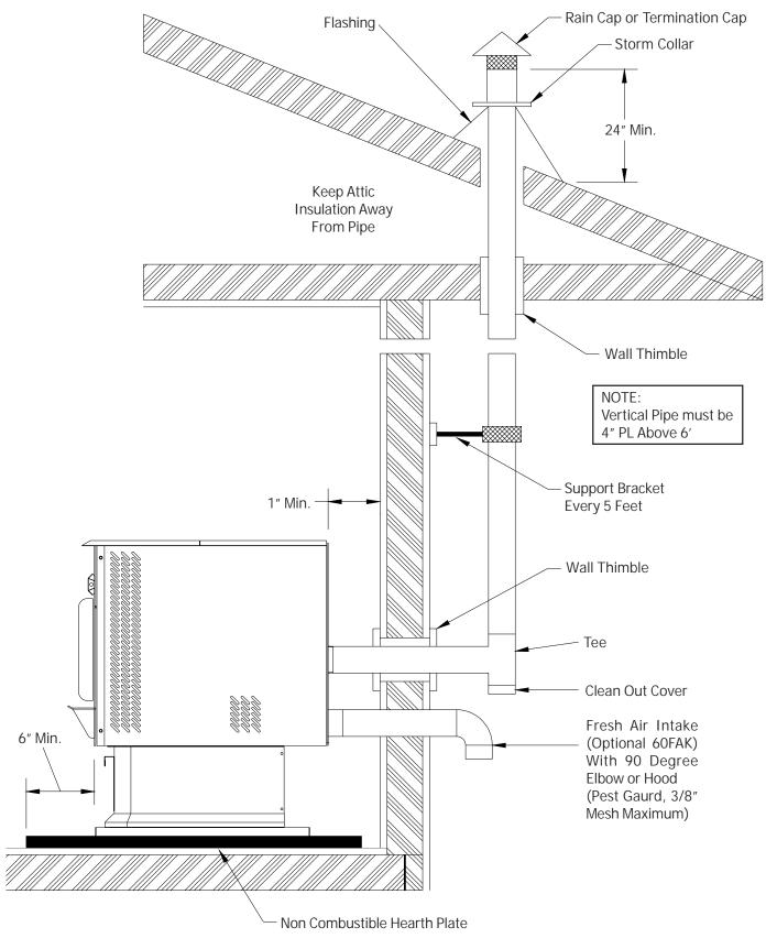
The Hearth Pad is not required under the unit if the floor is noncombustible but is required 6 inches (152mm) beyond the front of the unit and 6 inches (152mm) beyond each side of the door.
