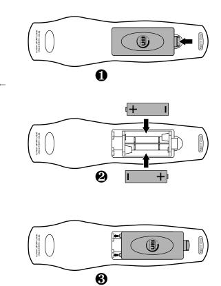
1. On the back of the remote control, push the tab and lift off the battery cover.
