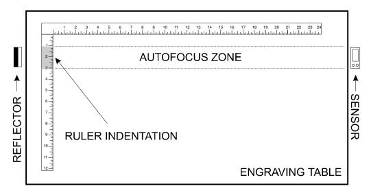
To clean these parts, dampen a soft cotton cloth with water and gently wipe across the reflective surface in one direction. **DO NOT** rub hard or create scratches in the plastic, otherwise the AUTOFOCUS system will malfunction. **DO NOT** use any type of cleaners, only use water or a light solution of hand soap and water on the sensor or reflector.
