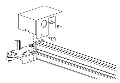
Inspect the #2 Mirror and clean it only if there is debris present. There are two ways to clean the mirror, with a moistened cotton swab or a moistened lens tissue.
