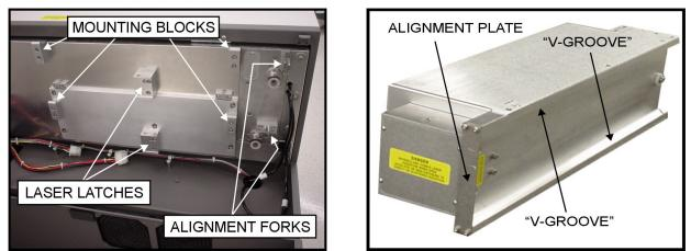
Open the Rear Cover and visually locate the Laser Mounting Block(s), the Laser Latch(es), and Alignment Fork(s). Notice that the Alignment Fork(s) have two plates, one small and one large. Locate the gap between the two plates.
