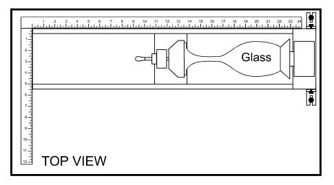
The Rotary Fixture is placed on the engraving table as the following diagram illustrates.
