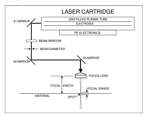
The laser cartridge receives power from the 48VDC power supply and its "trigger signal" from the CPU. When the laser system is power on and the trigger signal comes from the CPU, the RF electronics produce a 40 MHz signal across the electrodes located inside the plasma tube. This causes spontaneous photon emissions from the gas mixture that produces an invisible, infrared light beam at a frequency of 10.6 microns.
