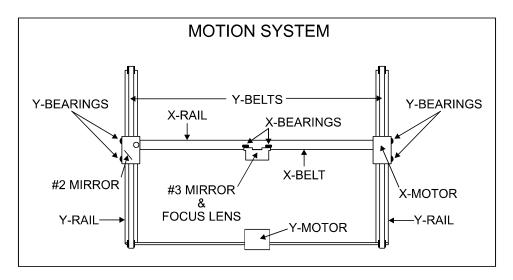
The CPU controls the movement of the motors, which moves the mirrors and focus lens across the engraving area and over the material. At the same time, it is synchronizing the laser pulses with the position of the focus lens. It is this precise positioning and timing of the laser pulses that produces the highest quality and fastest speed of engraving.
