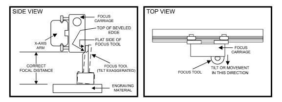
Remember, having the cursor, in the display, located on the tenths digit will move the table quickly and having it on the hundredths digit will move it more slowly. After focus has been established, remove the focus tool and press the "Z" button to move the focus carriage back into the home position.
