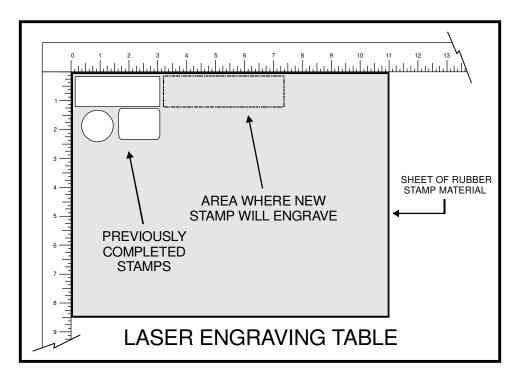
Place a sheet of rubber stamp material into the **UPPER LEFT CORNER** against the rulers, as the following diagram illustrates, and be sure to properly focus on the material. Now, set the printer driver settings as shown on the following page.
