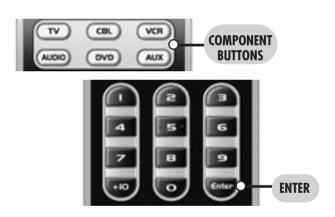
**STEP 2:** Press and hold the button you want to erase for two seconds. The component LED light will blink twice to confirm the erasure.
