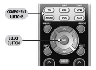
**STEP 5:** Point the AVEX R6 toward the component (in this example the TV) and punch in the first 3-digit code that you wrote down for that specific component. Use the Number buttons 0~9 on the remote to punch in the code. The TV LED light will blink each time a number is pressed.
