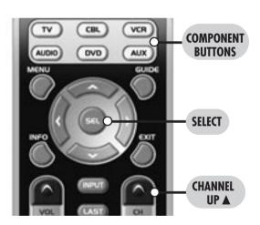
**STEP 3:** Press either the TV or CBL button that you want to use as the source of channel control. The component LED will blink three times to confirm it is saved.
