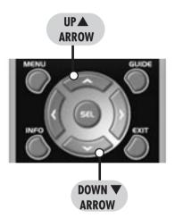
**STEP 3:** Point the AVEX R6 remote control toward the component and press the UP ▲ arrow (or DOWN ▼arrow) button once. Each time the UP or DOWN arrow button is pressed, the code will count up (or down) one code number and send a Power OFF signal. When the correct code is sent out, the component will turn off.
