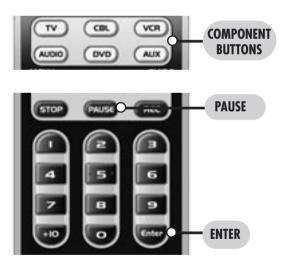
**STEP 3:** To exit Erase mode, press and hold both the component button and the ENTER (ENT) button at the same time until the component LED light blinks three times.
