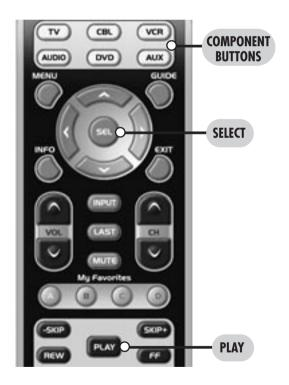
**STEP 3:** Press either the DVD or VCR button that you want to use as the source of Transport Control. The component LED will blink three times to confirm it is saved.
