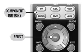
**STEP 2:** Press the VOLUME UP button and then press either the TV or AUDIO component button that you want to use for volume. The Component LED light will blink three times to confirm that it is saved. This sets up three buttons (Volume Up, Volume Down and MUTE) as a group for that component.
