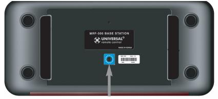
Slide off the mounting plate to reveal the RF ID# rotary switch. Use a small flat blade screwdriver to set the RF ID# to the address you used when programming the remote control (1-9 or A-F are valid addresses, while 0 is not a valid address).
