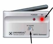
The RF LED lights when any RF signal is detected. If the RF LED flickers WITHOUT pressing a button on the remote control, you are receiving RF Interference and you must move the RFX-150 to another location. You can extend the wire up to 200' using standard CAT 5 cable. Place the RFX-150 in another room or crawlspace to avoid interference.
