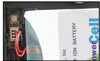
Battery Cable Plugged In
