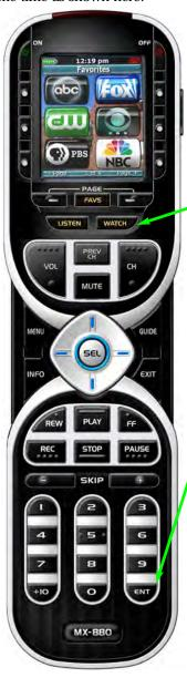
At the same time, press and hold both the WATCH button and the ENTER button. When the SETUP screen appears, you can release the two buttons.
