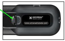
Note that the three contacts on the battery must connect to the three spring-loaded contacts in the MX-880. Angle the battery into the battery compartment, contacts first, then gently fit the rear of the battery into the compartment as well. Replace the battery cover by inserting the hinged end in first, then snapping the cover back into place.
