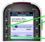
Use the DIM and BRIGHT buttons to adjust the lighting of the color screen.
