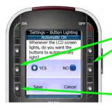
Use the YES and NO buttons to set the button back lighting to automatically turn on or not.
