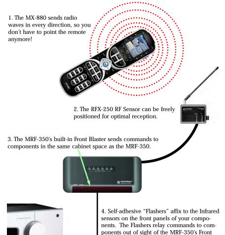
Blaster. The flashers plug in to the MRF-350's rear flasher line outputs via their 10 foot cables. Uniquely, the MRF-350 can also connect to components with rear panel IR Inputs
