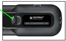
Note that the three contacts on the battery must connect to the three spring-loaded contacts in the MX-880Z. Angle the battery into the battery compartment, contacts first, then gently fit the rear of the battery into the compartment as well. Replace the battery cover by inserting the hinged end in first, then snapping the cover back into place.
