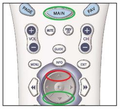
Press and Hold BOTH the MAIN and the DOWN thumbpad button at the same time to make it LIGHTER.
