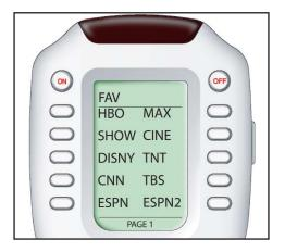
To EXIT Fav and return to the last activity/device selected, press the MAIN button ONCE. To EXIT Fav and go to the MAIN Menu, press the MAIN button twice.
