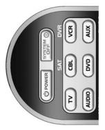
**STEP 2:** On the AVEX R6, press the Component button that you want to program (in this case the button that says TV) and the SELECT [SEL] button at the same time. Hold down both buttons for 2 seconds until the TV Component button light turns on. This signals that you are in programming mode.
