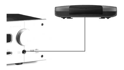
Self-adhesive "flashers" (included in the PowerBlaster™ kit) affix to the front panels of your Components. The flashers relay infrared commands to Components out-of-sight of the PowerBlaster's front blaster. The flashers plug into PowerBlaster's rear flasher line output jacks. Each flasher has a 10' cable to easily reach Components on nearby shelves.
