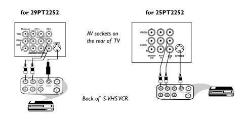
The S-Video connection on the rear of the TV is used for the playback of S-VHS VCR tapes, Video Discs, Video Games or Compact Disc-Interactive (cd-i) discs. Better picture detail and clarity is possible with the S-Video playback as compared to the picture from a normal antenna (RF) connection.
