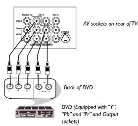
You can view the playback of DVD discs by using the COMPONENT VIDEO INPUT sockets on the rear of the TV.
