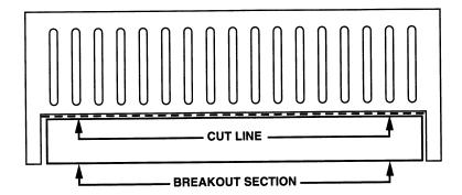
The breakout panel is removed by scoring the groove with a razor knife and bending the shaded portion away from the cut. The remaining edge can then be touched up with a small file. This allows the wiring to be run directly out of the control panel side of the amplifier.
