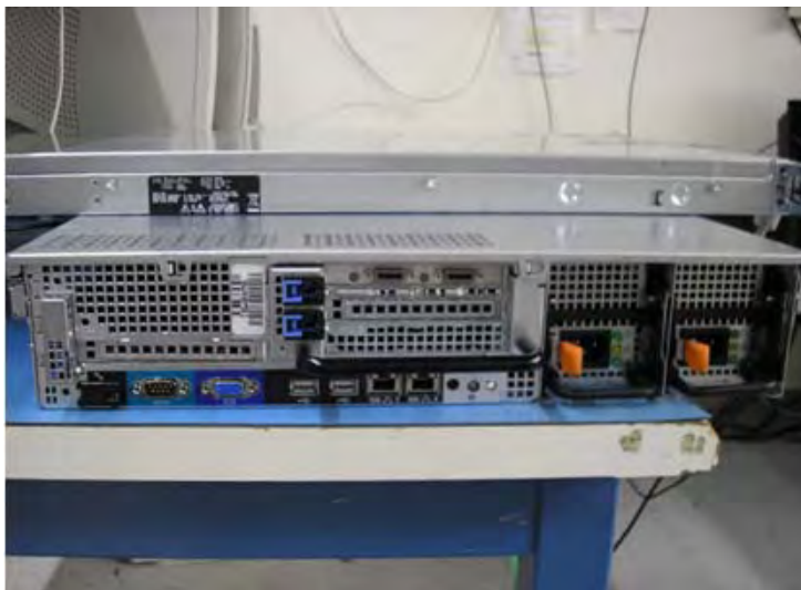
Figure 2. VOD 125/300W (Dell 2950 – Rear View)
