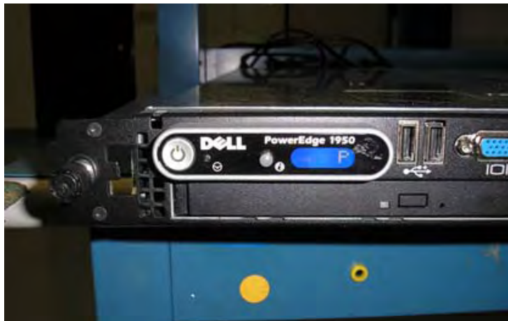
Figure 3. VOD 50W (Dell 1950 – Front View)
