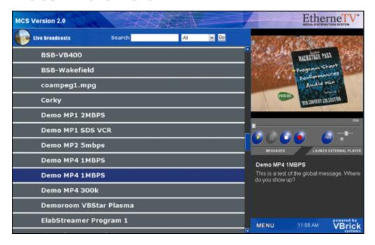
The Watch Television page enables a user to view live streams available on the network. The list of available streams are either live streams from a VBrick or another encoder or stored files that are multicast from an EtherneTV-NXG Video on Demand or other Video-on-Demand server.
