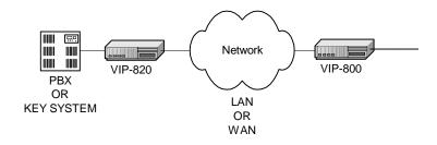
In this example, the VIP-810 and VIP-800 are connected to the data network as stand alone paging. This could be installed where network access is available, but not paging.
