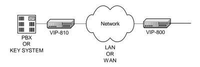
When using the VIP-800 with a PABX station port, a VIP-820 must be used to interface the telephone system with the network. When the PABX station port is accessed, the VIP-820 will activate the VIP-800.
